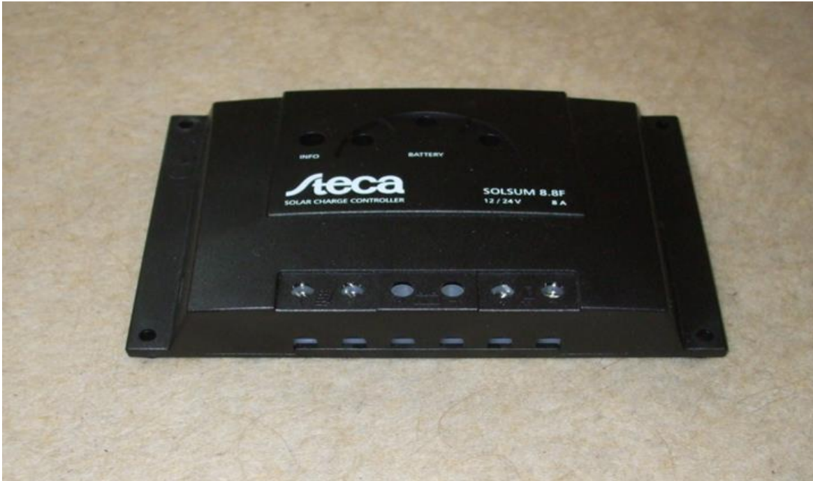
Peter's 8 amp charge controller. This magic box sits between the solar cell, and the load (battery and radio)
